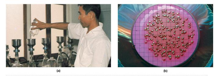
FIGURE 25.20 The membrane filter test for water purity. (a) Filtering water samples and trapping organisms on filter pads, which are then incubated. (Leon J. LeBeau/Biological Photo Service) (b) After incubation, the coliform colonies that appear are counted. (From Leboffe, M. J. and Pierce B.E., A PHOTOGRAPHIC ATLAS FOR THE MICROBIOLOGY LABORATORY, Fig. 8-11 978-0-89582-872-9, c 2011, Morton Publishing. Used with permission)
