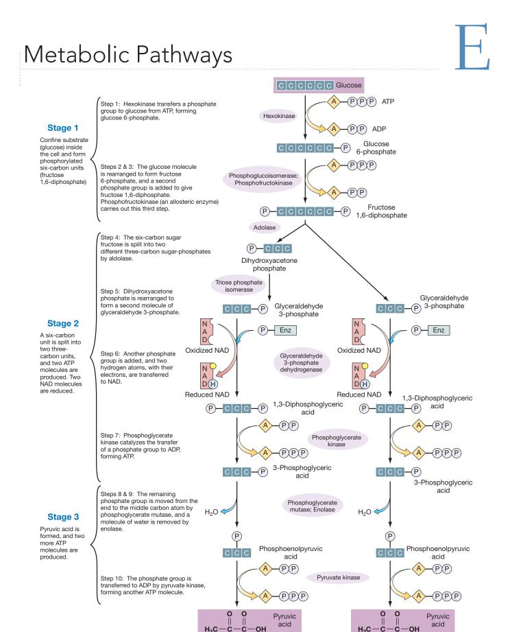
**FIGURE E.I Glycolysis (Embden-Meyerhof pathway).** Each of the 10 steps of glycolysis is catalyzed by a specific enzyme, which is indicated in a purple oval. (Refer to Chapter 5 for an explanation; Figure 5.11 shows a simplified version of the process. < p.124)
