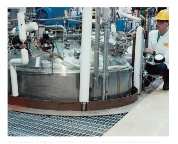
**FIGURE 26.18 Alcohol production.** Equipment for the industrial production of ethanol, using Zymomonas mobilis as a catalyst. (Courtesy Warren Gretz, National Renewable Energy Laboratory)
