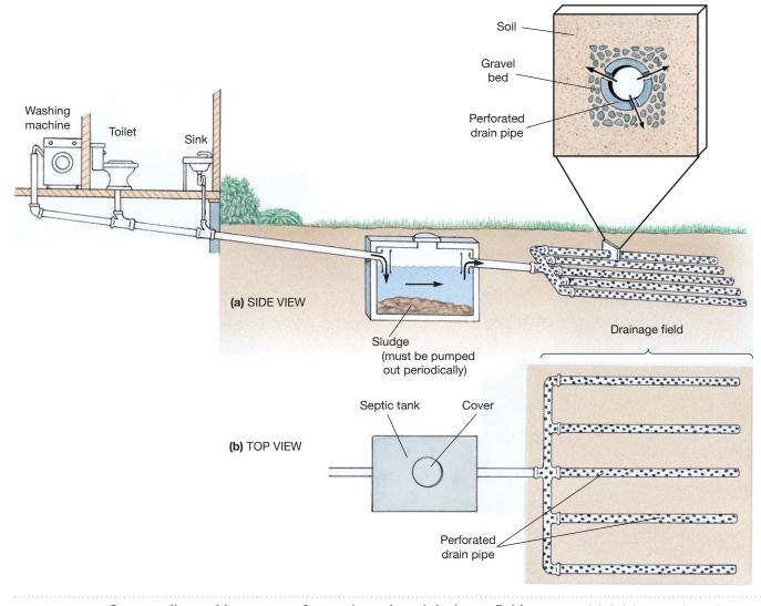
FIGURE 25.27 Sewage disposal by means of a septic tank and drainage field system. (a) Solid materials settle out as sludge, which undergoes microbial decay, while soluble materials continue to the drainage field. There (b) they seep out into the soil, which filters out bacteria and some viruses and binds phosphate. Soil bacteria decompose organic materials.
