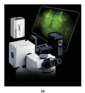
**FIGURE 3.19 (a)** A confocal microscope system manufactured by Olympus. Cell with microtubular fragments shown using **(b)** standard fluorescent microscopy, and **(c)** confocal microscopy. (*a*, *b*, *c*: Courtesy Olympus Corporation, Scientific Equipment Division)
