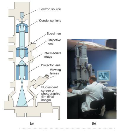
**FIGURE 3.21 Electron microscopy.** (a) A cross-sectional diagram of an electron microscope, showing the pathways of the electron beam as it is focused by electromagnetic lenses. (b) A modern scanning electron microscope in use. (b: ©Inga Spence, I/Visuals Unlimited/©Corbis)
