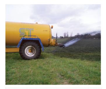
FIGURE 25.26 Sludge digestion. The spraying of municipal sewage sludge into farmland is designed to return nutrients to the soil. But if treatment is not complete, it may also add pathogens to the soil. (Robert Brook/Photo Researchers, Inc.)
