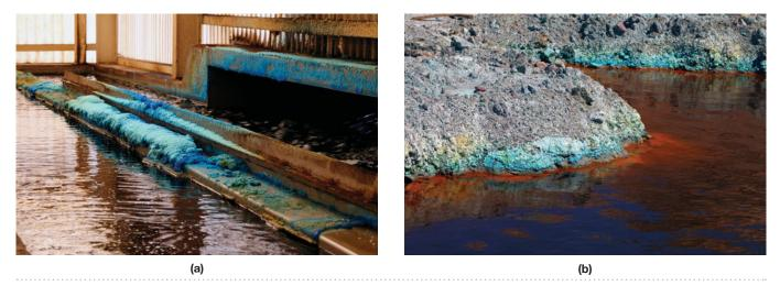
**FIGURE 26.21 Microbial mining.** Mining is made easier in many places by the activity of microorganisms. (a) Bacterial copper ore processing. Water flowing into a bioleaching bath, where copper is extracted from concentrated solutions of copper sulphide ores. (b) Copper mine collecting pond, with copper mineral deposits (blue) around its edges. (*Dirk Wiersma/Photo Researchers*)
