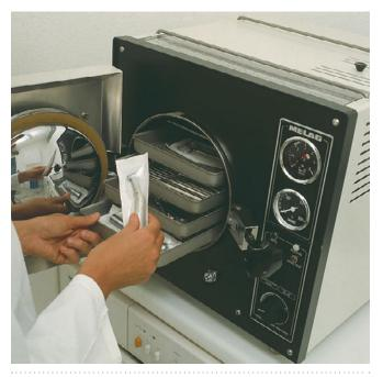
FIGURE 12.8 Hot-air oven used for sterilizing metal and glass items. (Ulrich Sapountis/Okapia/Photo Researchers, Inc.)
