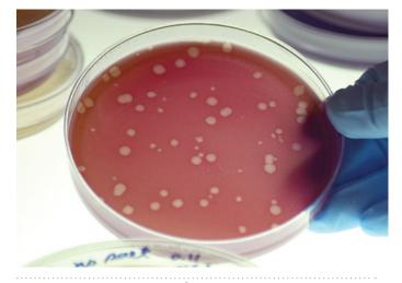
**FIGURE 25.22 Easyphage**<sup>(®)</sup>. This test uses bacteriophages to indicate the presence of coliform bacteria in food or water testing. Presence of a plaque (hole) is a positive indicator of a specific bacterium which has been grown on the Petri dish. This means that this bacterium was present in the original food or water sample; otherwise bacteriophages which attack it would not be present. (*Courtesy Scientific Methods, Inc.*)
