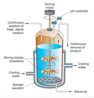
**FIGURE 26.16 A continuous reactor.** Fresh culture medium is introduced on one side, and medium containing product is withdrawn at the other side in a continuous process.
