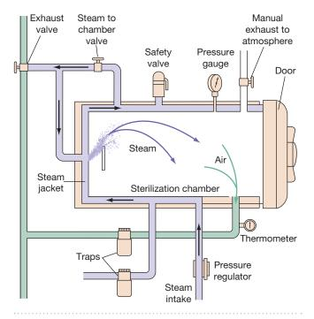
FIGURE 12.10 The autoclave. Steam is heated in the jacket of an autoclave, enters the sterilization chamber through an opening at the upper rear, and is exhausted through a vent at the bottom front.
