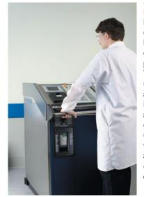
FIGURE 12.6 Vaporized hydrogen peroxide (VHP) disinfection. The low-temperature VHP process is fully controlled, repeatable, and easily validated. This "dry" process operates under low concentration and is highly efficacious. It is fast and compatible with a wide range of surface and component materials. It is used worldwide for sterility testing in isolators, rooms and other sealed enclosures. (Photo of VHP(R) 1000 Mobile courtesy of STERIS Corporation)
