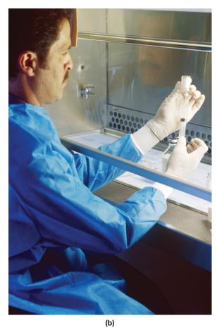
FIGURE 25.10 Measuring airborne microbes. (a) An air-sampling device used to measure airborne bacteria and fungi. (*Courtesy Graseby Andersen, Inc.*) (b) Technicians are protected from the airborne spread of organisms by the use of a laminar flow hood, which suctions air away from the opening and filters it before expelling it. (*Will & Deni McIntyre/Photo Researchers*)
