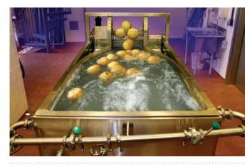
FIGURE 26.3 Surface pasteurization of cantaloupes. At the rear, cantaloupes are being lifted out of the bath following a 3-minute immersion at 169°F. (Courtesy Bassam A. Annous, USDA-ARS Food Safety Intervention Technologies Research Unit, Wyndmoor, PA)
