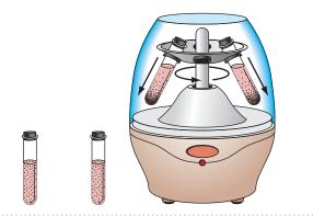
**FIGURE 4.8 A centrifuge.** Suspended particles in tubes of liquid are whirled around at high speeds, causing them to settle to the bottom of the tubes or to form bands at different levels. The rate of settling or the locations of the bands can be used to determine the size, weight, and shape of the particles. Band locations are given in Svedberg (S) units.
