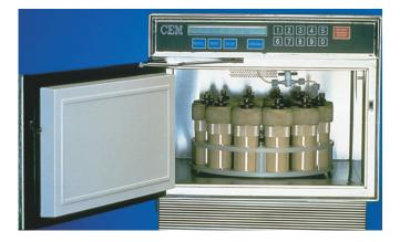
**FIGURE 12.17 Microwave sterilization.** The MikroClave<sup>TM</sup> system is specifically designed for rapid sterilization of microbiological media and solutions. Using microwave energy, it can sterilize 1.2 liters of media in 6.5 minutes, or 100 ml in 45 seconds. Agar need not be boiled prior to sterilization. (*CEM Corporation*)
