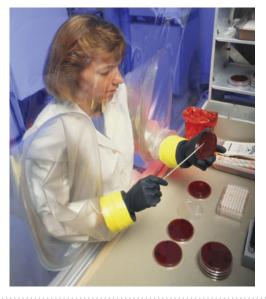
FIGURE 6.24 Anaerobic transfer. A large transfer chamber with an air lock for introducing equipment and cultures and with ports to allow manipulation of the cultures. (Hank Morgan/ Photo Researchers)
