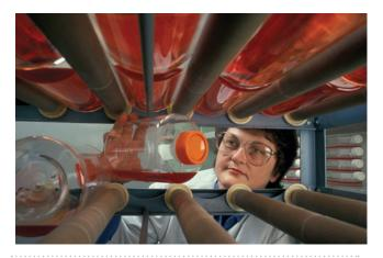
**FIGURE 10.20** A view from the end of a bottle lined with spiral plastic coils. One way to increase cell density is by increasing the surface area to which cells can attach. The bottle is rotated slowly at about 5 rev/h, so that a small volume of culture fluid can be used. Cells tolerate being out of the culture fluid for short periods. (Keith Weller/Courtesy USDA)
